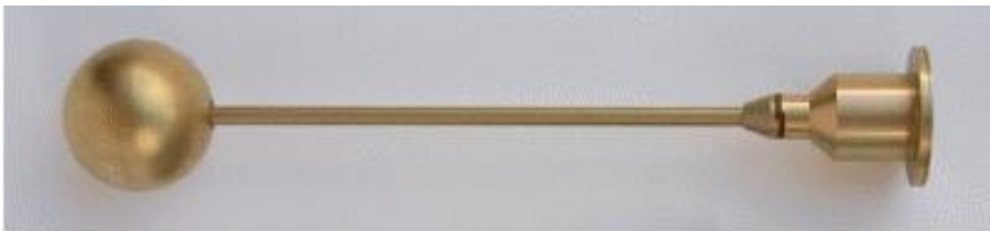
Figure 5.1: A Langmuir Probe. Source: http://www.space.irfu.se , September 12, 2007.
