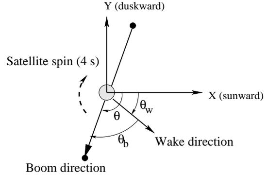
Fig. 6. Angles in the spacecraft spin plane:  $\theta_b$  – angle between the boom and the direction of the wake fbw,  $\theta_w$  – angle between the positive  $X_{GSE}$  direction and the wake,  $\theta$  – angle between the positive  $X_{GSE}$  direction and the boom.
