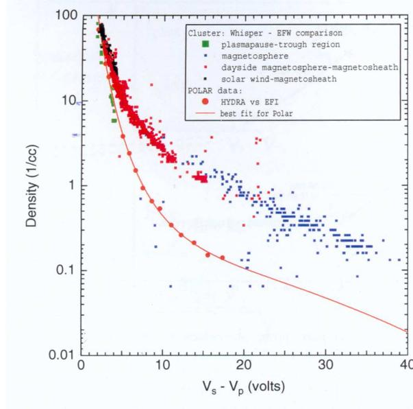
Figure 4.1: Spacecraft potential-density relation for the Cluster spacecraft. (Adapted from *Pedersen et al.* (2001)).
