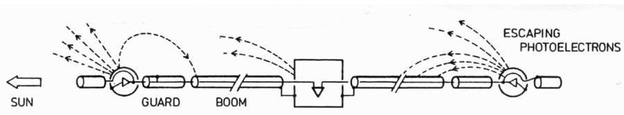
Figure 3.5: The probe furthest away from the Sun will lose more photoelectrons to the positively charged booms than the probe close to the Sun, which will cause a spurious sunward electric field. The errors can be decreased by applying a negatively biased guard near the probes. (Adapted from Pedersen *et al.* (1984).)
