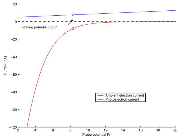
Figure 3.2: Current balance of impinging plasma electrons and escaping photoelectrons to a probe of radius 4 cm. The temperature of the plasma is 10 eV and the density is  $10 \text{ cm}^{-3}$ . The photoelectron current density is  $6 \text{ nAcm}^{-2}$ . In such a tenuous plasma the ion current is negligible. The floating potential is around 8.3 V.
