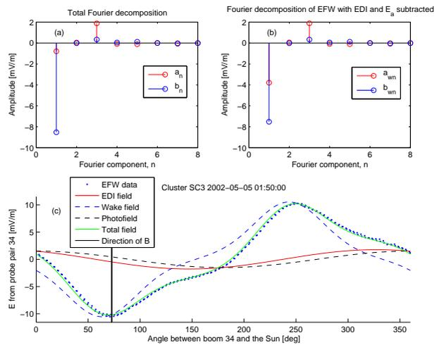
Fig. 7. Fourier decomposition of one spin for wake affected EFW data from 2002-05-05 01:50:00 for probe pair 34 on spacecraft 3. Panel (a) shows the complete decomposition of the spin, while panel (b) displays the Fourier decomposition with the background electric field from EDI and the sunward offset field subtracted. In panel (c) the data (blue) is shown together with the complete Fourier decomposition (red), the EDI field (blue),  $E_a^0 \cos \theta$  (black), and the wake field (green).
