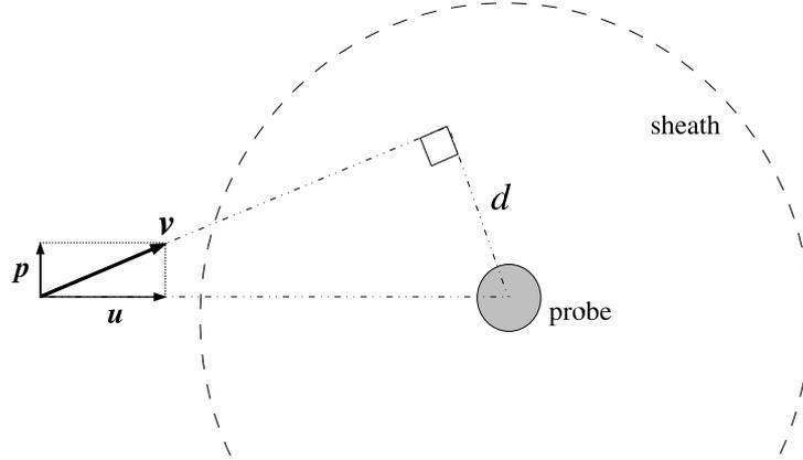
Figure 3.1: *Probe in a flowing plasma.* The velocity outside the sheath is  $v$ , which can be decomposed into the radial component  $u$  and the tangential component  $p$ . The sheath is assumed to be much larger than the probe.  $d$  is the impact parameter.
