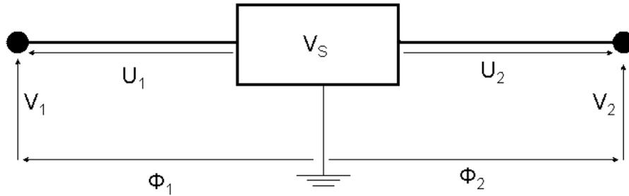
Figure 3.3: Simplified electrical schema of the double-probe/spacecraft system.  $U_1$  and  $U_2$  are the potentials between spacecraft and probes,  $V_1$  and  $V_2$  the potentials between probes and plasma and  $\Phi_1 - \Phi_2$  the real potential difference in the plasma. The ground point is of course arbitrary.
