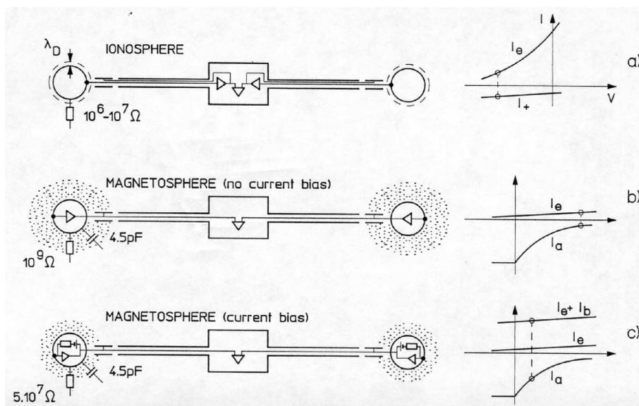
Figure 3.4: The double-probe instrument in different environments: a) The ionosphere, b) The magnetosphere, c) The magnetosphere with bias current. The bias current brings the probe potential closer to the plasma potential, where small spurious currents will not influence the potential of the probe. (Adapted from *Pedersen et al.* (1998))
