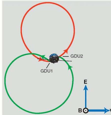
Figure 5.3: The Electron Drift Instrument uses the drift of electrons in a magnetised plasma to measure the electric field. Two high energetic electron beams are emitted from the spacecraft to measure the drift. (Adapted from *Paschmann et al.* (2001)).
