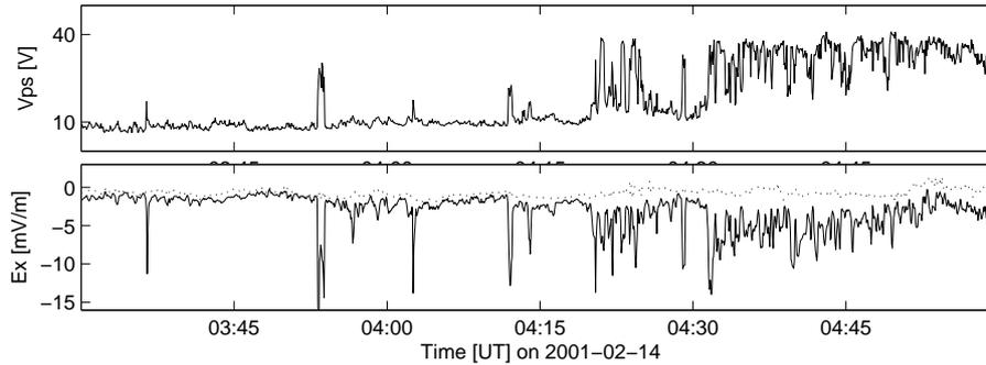
Fig. 1. EFW and EDI electric field data from Cluster 1. The top panel shows the spacecraft potential  $V_s$ , while the lower panel displays the EDI (dashed line) and EFW (solid line) estimates of the GSE  $X$  component of the electric field. Strong discrepancies between the EDI and EFW electric field estimates can be seen when  $V_s$  is high. At the time of observation Cluster was above the northern polar cap at  $(-2.5, 1.4, 4.9) R_E$  in GSE coordinates.
