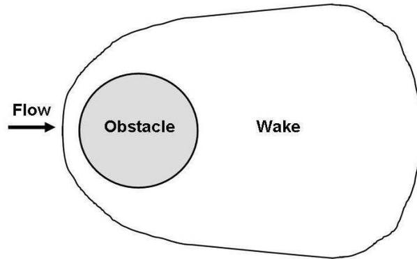
Figure 4.3: Schematic picture of an *enhanced* wake. The ions are deflected by the positive potential of the spacecraft, which is higher than the kinetic energy of the ions ( $eV_s > E_k^i$ ). As for the wake in figure 4.2, this wake will be negatively charged, if the electrons are subsonic.
