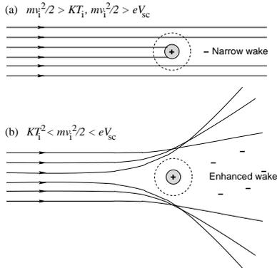
**Figure 4.** Sketch of wake formation in supersonic flows. (a) Narrow wake. (b) Enhanced wake.
