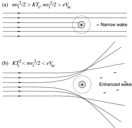
FIG. 1: Sketch of wake formation in mesosonic flows. (a) For ion flow energies higher than the spacecraft potential,  $V_{sc}$ , the wake has the typical transverse size of the spacecraft (narrow wake case). (b) For ion flow energy below  $V_{sc}$ , ions will scatter off the positive electrostatic potential from the spacecraft, creating an enhanced wake.
