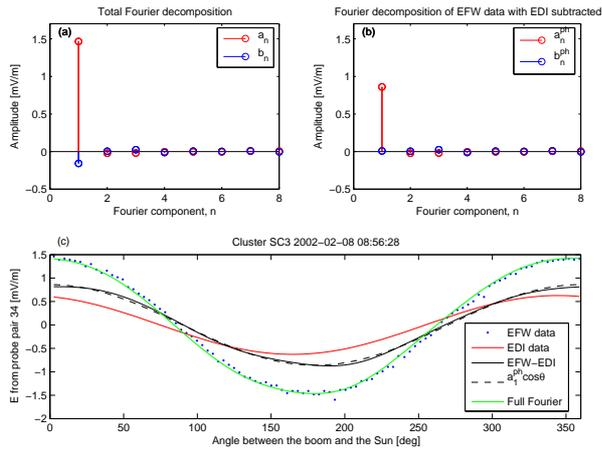
Fig. 4. Fourier decomposition of one spin from 2002-02-08 08:56:28 for probe pair 34 on spacecraft 3. Panel (a) shows the complete decomposition of the spin, while panel (b) displays the Fourier decomposition with the background electric field from EDI subtracted. In panel (c) the data (blue dots) is shown together with the complete Fourier decomposition (green), the EDI field (red), the resulting field from (b) (solid black) and  $E_a^0 \cos \theta$  (dashed black).
