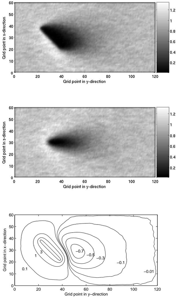
FIG. 3: Averaged results from the boom simulation between  $30 \omega_{pe}^{-1}$  and  $60 \omega_{pe}^{-1}$ . (The grid spacing is 4 m.) (a) Ion density in the  $x - y$ -plane through the boom. (b) Ion density in the  $y - z$ -plane through the boom. (c) Potential in the  $x - y$ -plane cutting the boom. The minimum value of the potential in the wake is  $-0.80$  V. Equipotential contours are given at  $-0.7$ ,  $-0.5$ ,  $-0.3$ ,  $-0.1$ ,  $-0.01$ ,  $0.1$ ,  $1$ ,  $5$ , and  $10$  V.
