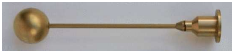
Figure 5.1: A Langmuir probe. Figure from www.space.irfu.se/rosetta/galleri.html .
