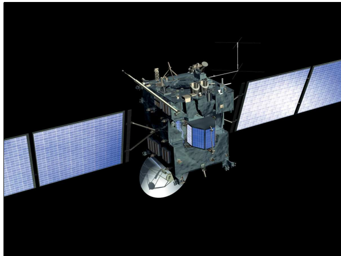
Figure 11: A fully equipped Rosetta with the HGA completely unfolded. Facing the viewer is the -x side with the small lander mounted and the LAP 1 boom, LAP 2 is missing in this model. (from http://esamultimedia.esa.int/images/Science/ )
